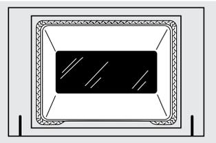
The gasket is designed with a gap at the bottom to allow for proper air circulation. Do not rub or clean the door gasket—it has an extremely low resistance to abrasion. If you notice the gasket becoming worn, frayed or damaged in any way or if it has become displaced on the door, you should have it replaced.
