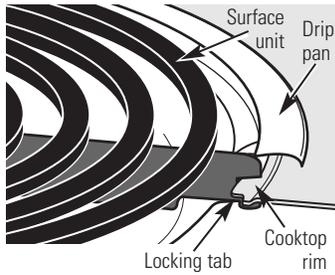
When properly seated, the locking tab should lock onto the cooktop rim through the notch in the drip pan.
