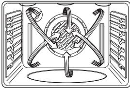
In a convection oven, a fan circulates hot air over, under and around the food. This circulating hot air is evenly distributed throughout the oven cavity. As a result, foods are evenly cooked and browned – often in less time than with regular heat.
