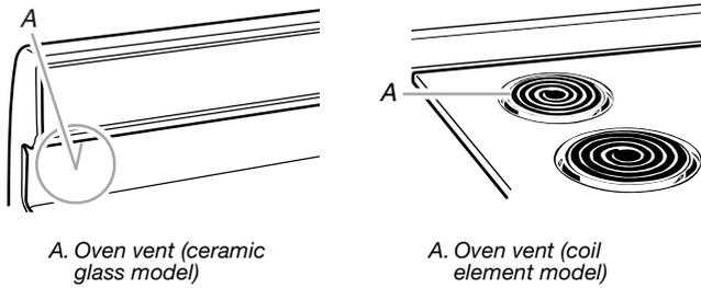
The oven vent releases hot air and moisture from the oven, and should not be blocked or covered. Blocking or covering the vent will cause poor air circulation, affecting cooking and cleaning results. Do not set plastics, paper or other items that could melt or burn near the oven vent.
